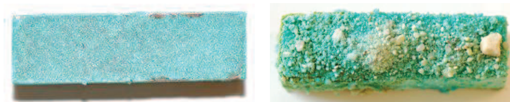
Fig. 1. Sample (No. 3) with model corrosion layer created in hydrochloric acid (left) and sample (No. 6) with corrosion layer created in hydrochloric acid with addition of sand (right).
